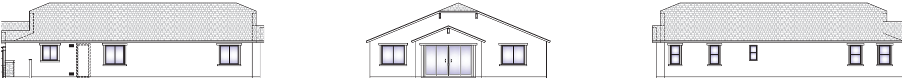
4 OPT. EXTENDED COVERED PATIO LEFT, REAR & RIGHT @ ELEVATION B SCALE: 1/8" = 1'-0" REAR & LEFT ELEVATIONS DO NOT CHANGE WITH THIS OPTION REF. A2.2 SHEETS FOR ADDITIONAL NOTES & DIMENSIONS
