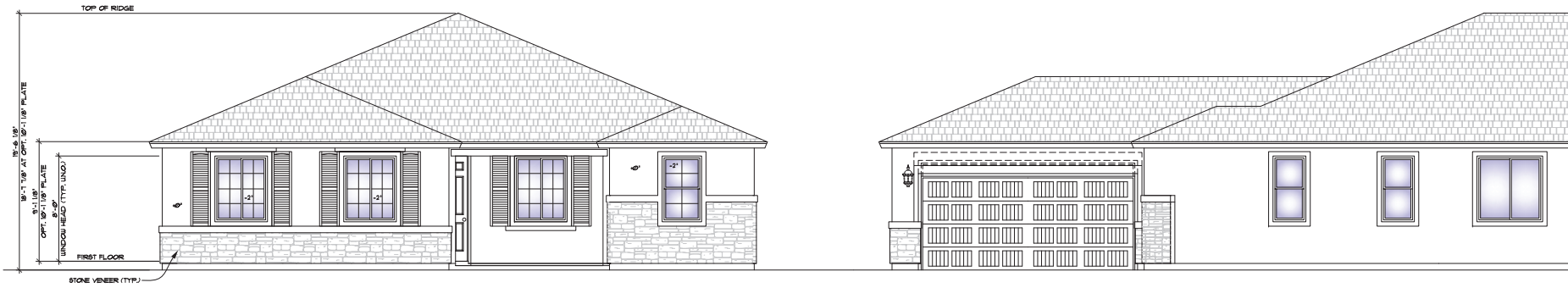
5 OPT. GUEST SUITE FRONT & RIGHT @ ELEVATION C SCALE: 1/4" = 1'-0" REAR & LEFT ELEVATIONS DO NOT CHANGE WITH THIS OPTION RE: A23 SHEETS FOR ADDITIONAL NOTES & DIMENSIONS
