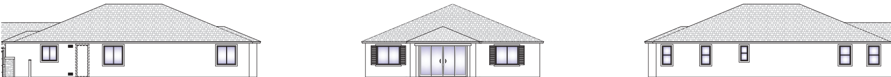
5 OPT. EXTENDED COVERED PATIO LEFT, REAR & RIGHT @ ELEVATION C SCALE: 1/8" = 1'-0" REAR & LEFT ELEVATIONS DO NOT CHANGE WITH THIS OPTION REF. A2.3 SHEETS FOR ADDITIONAL NOTES & DIMENSIONS
