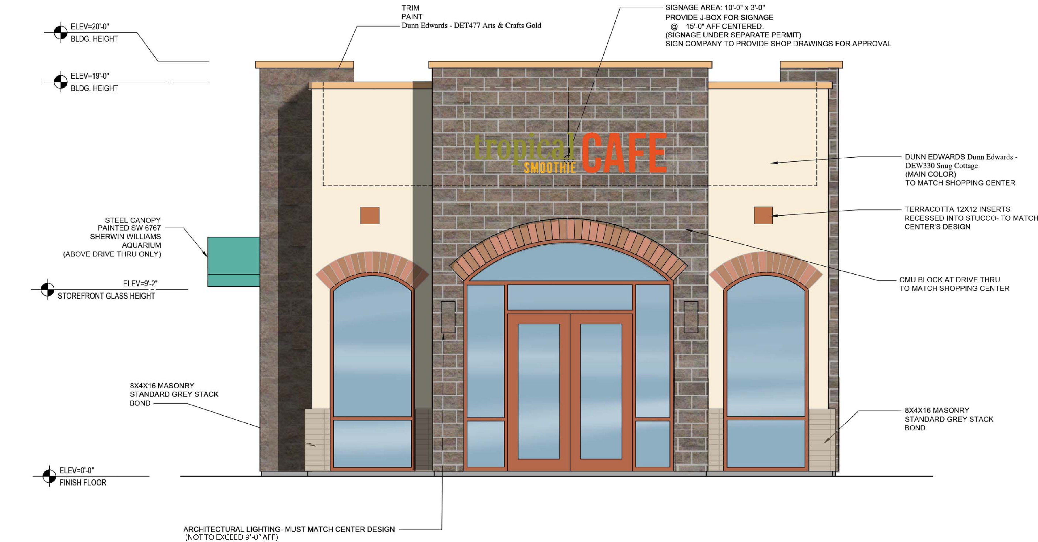
2 (EAST) FRONT BUILDING ELEVATION SCALE: 3/8" = 1'-0"
