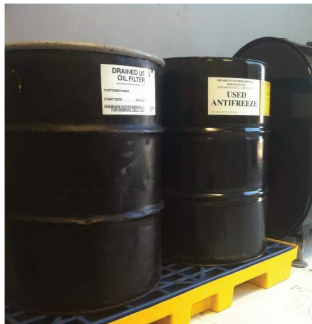
These waste containers are a good example of clear labeling and covered storage.
