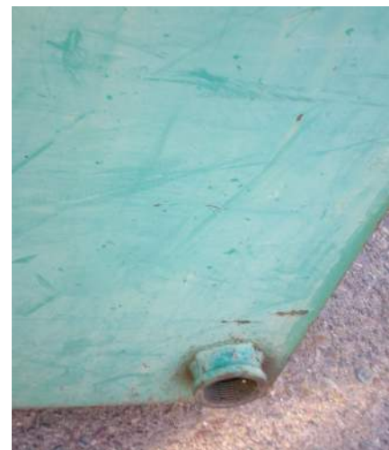
Dumpsters must be watertight. If there is a drain, it must be plugged.
