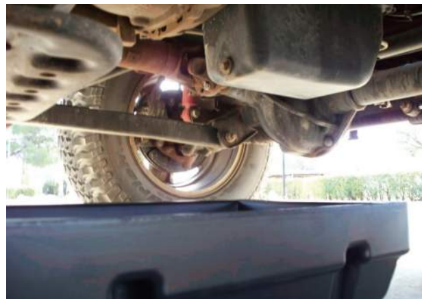
Use drip pans or absorbent pads under equipment during maintenance that involves fluids.
