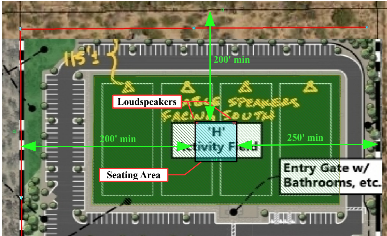
Figure 3.3. Loudspeaker Placement for Outdoor Services
