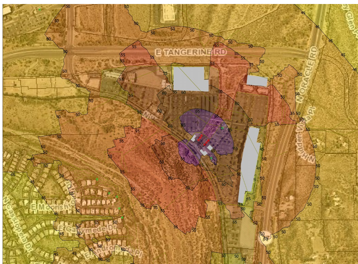
Figure 3.7. Adjusted 63 Hz Sound Pressure Level Contours - Courtyard with PA
